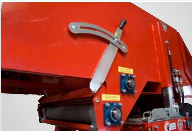
Material output exact adjustable through a slide valve
