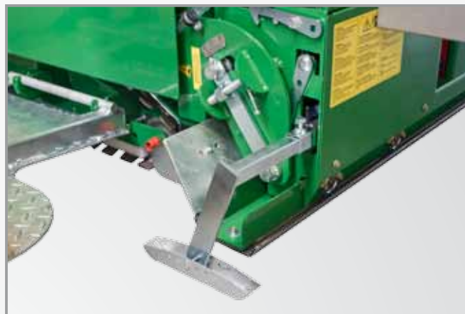
Integrated height leveling for evenly flat installation
