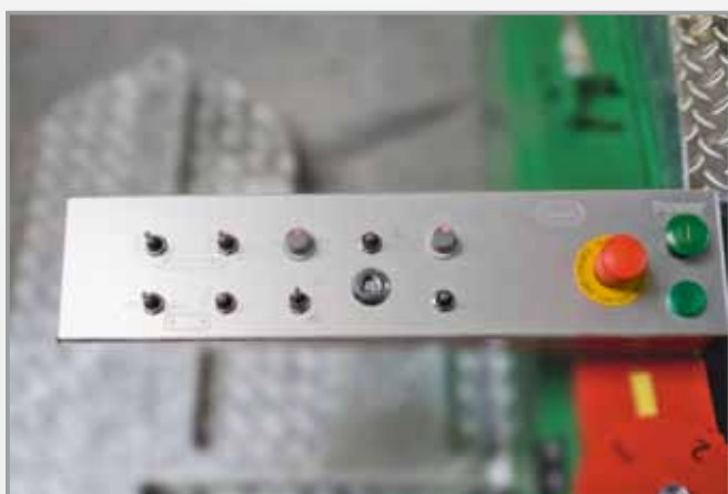
Ergonomic control panel, installed on both sides
