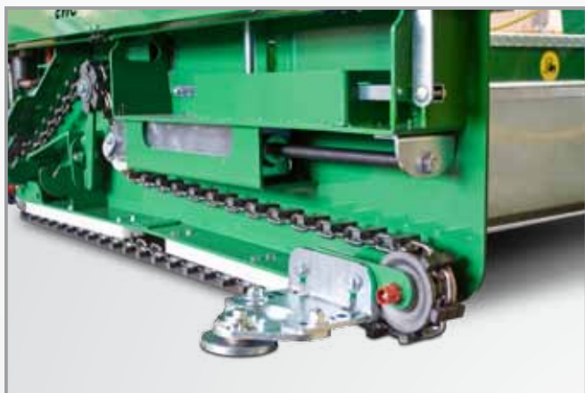
Repulse wheel for the installation alongside border stones
