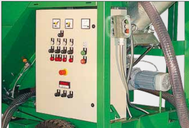
Switch cabinet with central electrical control
